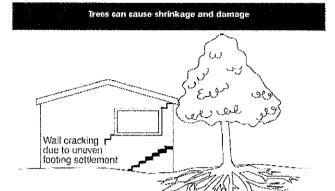
As the weather pattern changes and the soil begins to dry out, the external footings will be first affected, beginning with the locations where the sun's effect is strongest. This has the effect of lowering the external footings. The doming is accentuated and cracking reduces or disappears where it occurred because of dishing, but other cracks open up. The roof lines may become convex.
